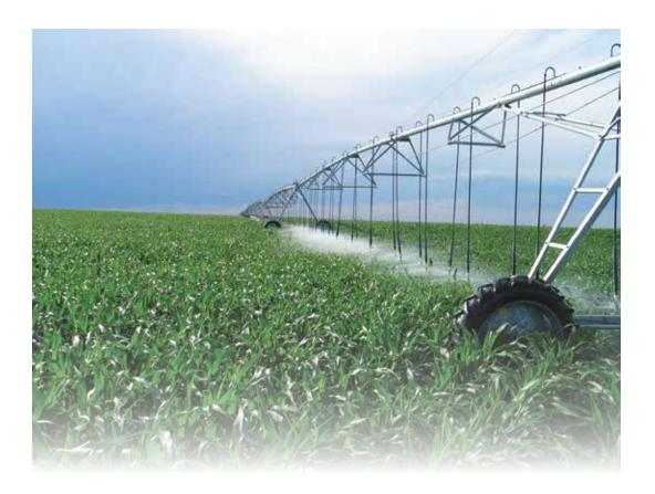
istorically, farmers along the west coast have never considered center pivots efficient irrigation systems. Drip systems have always been a popular option in the region due to their low flow rates and high application efficiency.
